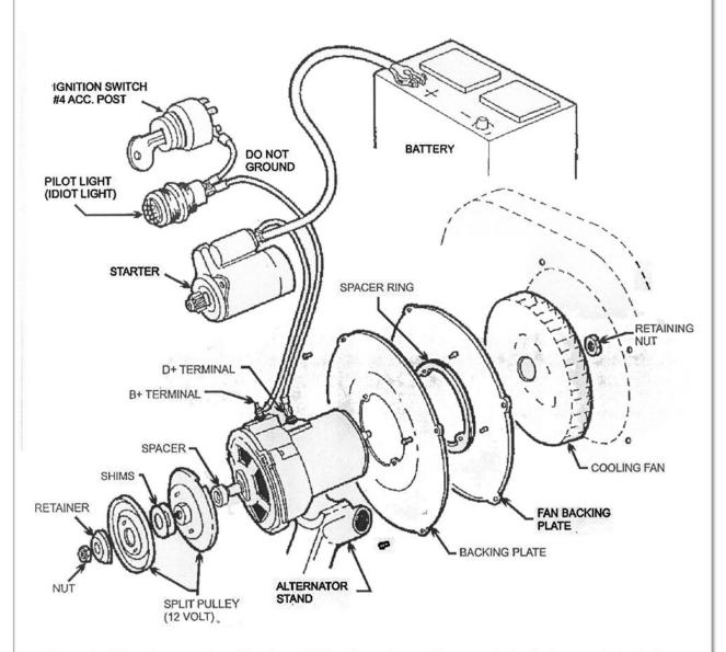
Generator/Alternator swap in a 12 volt car. At the alternator, small green wire to D+, large red wire to B+. Under the rear seat, remove the regulator and splice - small green wire to small blue wire: (generator light), large red wire from alternator to other red wires, (ignition switch lead and + battery lead). Generator dash light must work or alternator will not charge.
